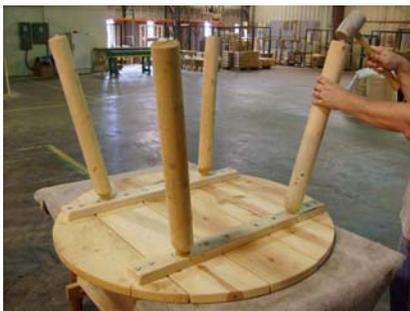
1. Insert table legs into pre-drilled holes in table top underlay. Use rubber mallet to tap any doweled ends into place. If using a hammer, be sure to pad impact area to avoid damaging the product.
