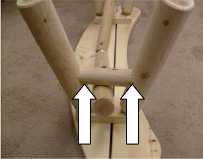
11. Use 2” screws to secure the 8 ½” leg braces to the bench legs, as identified by arrows in photo.
