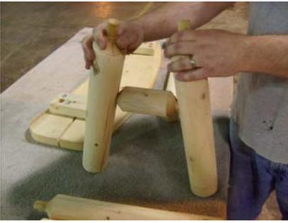
6. Insert 8 ½” leg braces into pre-drilled holes on bench legs to join legs and create leg assembly. Use mallet to tap them into place. *Note: Newer table models will utilize 8 ½” braces which recess into holes on table legs.*
