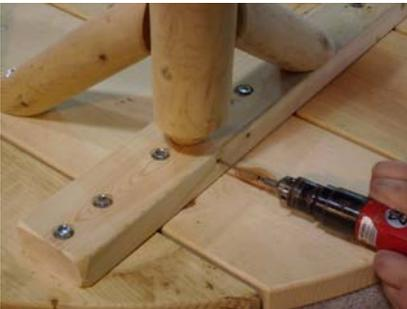
4. Use 2 ½” screws to secure the doveled end of the table legs to the table underlay.
