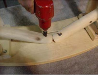
8. Install 18” seat brace (as shown in next two photos). Center the angled brace ends in middle of the bench. Place the other end of the brace underneath the 8 ½” leg brace. Insert the 2 ½” lag bolts to secure the seat braces to the seat bottom.
