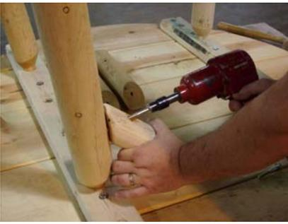
2. Use 2 ½” lag bolts to secure 11” leg braces to the table legs, as well as to bottom of table (as shown in these two photos).
