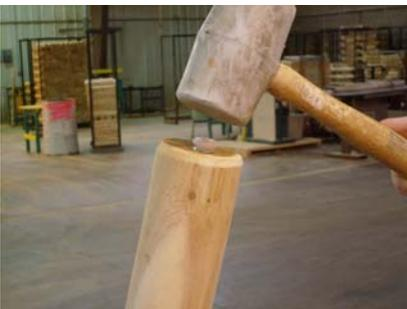
5. Use rubber mallet or hammer to tap leveling glides into bottom of each table leg.
