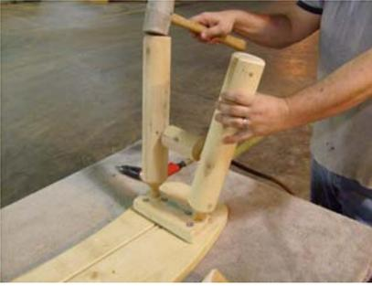
7. Tap all bench leg assemblies into the pre-drilled holes on the bottom of the bench.
