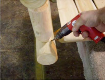
5. Install 2" screw where all doweled ends were inserted, securing seat and seat back to arm assemblies.
