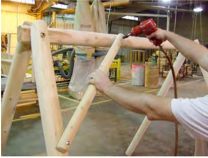
8. Stand frame upright and tighten 7 ½” machine bolts *only enough* to allow frame to stand freely. Measure 24” down from top of the swing leg, and 24” out from end of top pole. At these points, use 4” lag bolts to secure the remaining four braces to the swing (as shown in these two photos). Use ¼” washer when inserting each lag bolt. Now, tighten 7 ½” machine bolts firmly.
