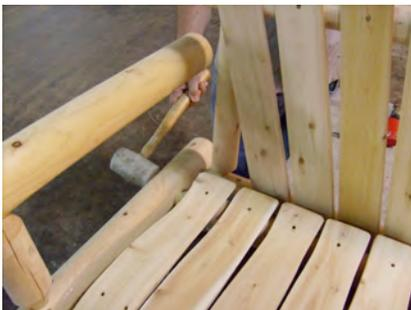
2. Attach pre-assembled seat back to remaining holes at the rear of arm assemblies. Tap arms into place with rubber mallet or hammer.
