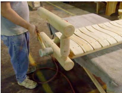
1. Attach both swing arm assemblies to swing seat. Align the two doweled ends of swing seat with the two holes in the swing arm assembly. Tap arms into place using rubber mallet or hammer. If using a hammer, be sure to pad impact area to avoid damage to the product.
