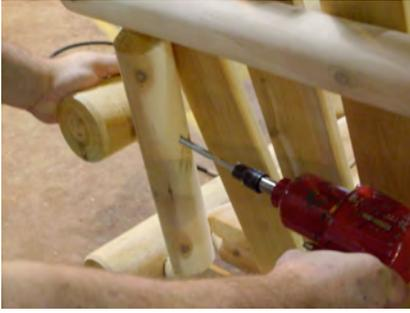
3. Through pre-drilled holes in seat back, use 3 3/8" lag bolts to secure the arms to the seat back (as shown). Use a 5/16 washer when inserting each 3 3/8" lag bolt.
