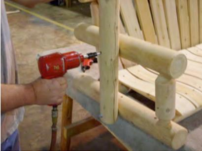
4. Attach swing hangers to arm assemblies using 5" lag bolts. Align pre-drilled holes on swing hanger with pre-drilled holes on swing arm assemblies (both upper and lower arms).
