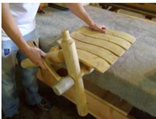
2. Attach leg assemblies to dowels on both sides of pre-assembled seat (as shown). Use rubber mallet to ensure secure fit. If using a hammer, be sure to pad impact area to prevent damage.
