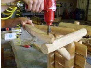
8. Lay the Rocker on its side and align the pre-drilled holes of the rocker runner so they are centered on the front and back legs. *Note: The bottoms of the front and back legs should not extend below the bottom of the rocker runner.* Attach rocker runners to legs using 3 3/8" lag bolts (as shown in both photos).
