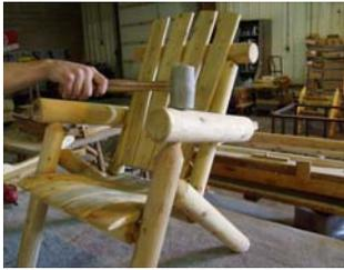
4. Attach both arm pieces to exposed dowels on the leg assemblies (as shown). At this point, set Rocker on a flat surface to ensure that all components are aligned and the Rocker is level. Use rubber mallet or hammer (with padding) to ensure all dowels are secure in each receiving piece.
