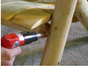
5. Using 2" screws, secure all doweled points (as shown in photo series). Repeat process for both sides of Rocker.
