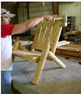
3. Insert doweled ends of pre-assembled seat back into the holes at the rear of the seat assembly. If doweled ends do not line up, gently tap seat back sidepieces in or out as needed. Tap top of seat back with rubber mallet or hammer (with padding) to ensure secure fit (as shown).
