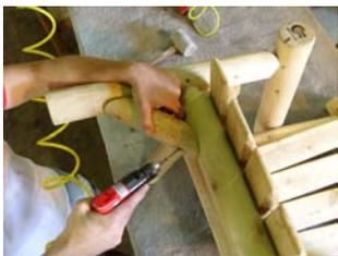
7. Use 2 1/2" screws to attach each 9" brace to front of seat bottom and to the leg assembly (as shown).
